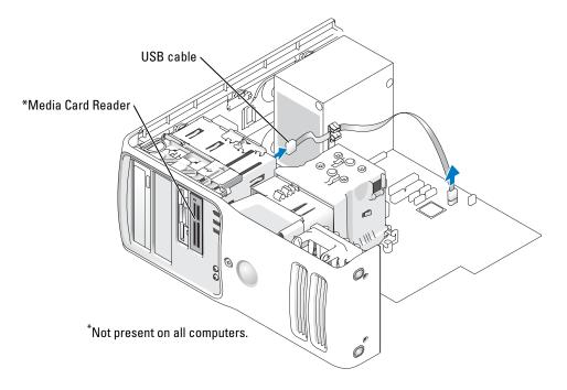
5 Disconnect the USB cable on the back of the Media Card Reader to the front panel USB connector on the system board (see page 71) and route the cable through the clip on the shroud.
